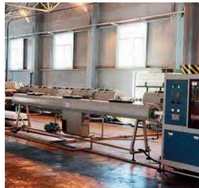
Production line of pipes with a diameter of 90, 110, 160 and 200mm. It is also possible to make a profile pipe with sizes of 60x60 and 80x100 with thickness of a wall 5 and 7 mm. Productivity of this line is 2500 kg per day.
